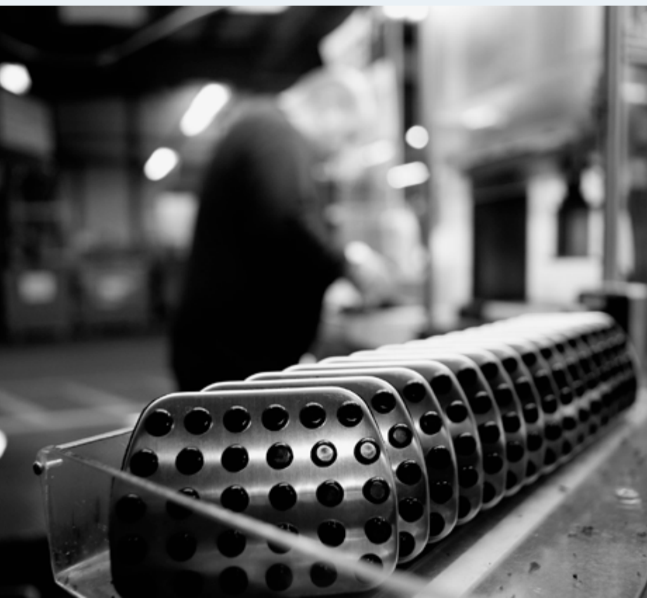
Rubber pedal covers are produced with and without a metal composite.
